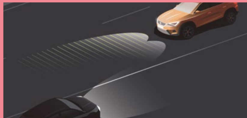
High Beam Assist This system automatically switches headlights between low and high beam when detecting a vehicle ahead, reducing dazzle to other drivers to support safer driving.
