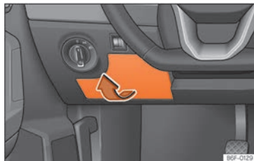
Fig. 160 On the dashboard on the driver side: lid of the fuse box.
