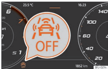
Fig. 112 On the screen of the instrument panel Front Assist switched off message.
