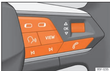
Fig. 13 Right side of multifunction steering wheel: buttons to the menus and informative indications on the instrument panel (depending on the version).
