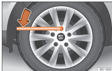
Fig. 189 Tyre change: slacken the wheel bolts.
