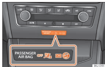
Fig. 31 Centre of the instrument panel: control lamp for deactivated front passenger airbag in centre console.
