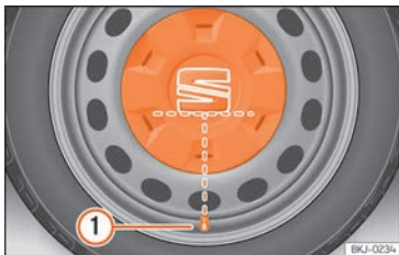
Fig. 185 Correct positioning of the central wheel trim for steel rims.
