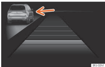
Fig. 107 On the instrument panel display: ACC active, vehicle detected on the left.
