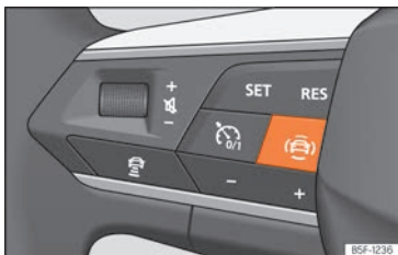
Fig. 96 Left side of the multifunction steering wheel: button for driver assistance systems [depending on the version].
