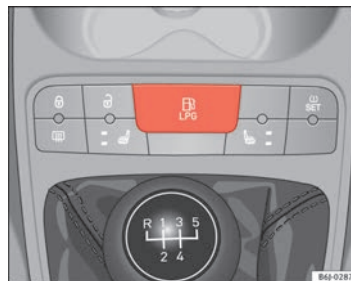
Fig. 108 Centre console: gas system control switch.
