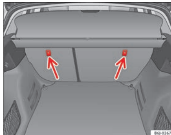
Fig. 27 Position of the Top Tether rings on the back of the rear seat
