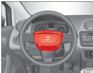
Fig. 16 Driver airbag located in steering wheel
