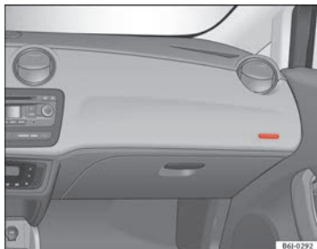
Fig. 17 Front passenger airbag located in dash panel
