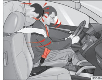
Fig. 9 The unbelted passenger in the rear seat is thrown forward violently, hitting the driver wearing a seat belt
