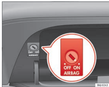
Fig. 21 In the glove compartment: switch for activating and deactivating the front passenger airbag
