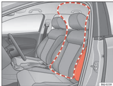
Fig. 20 Side airbag in driver seat
